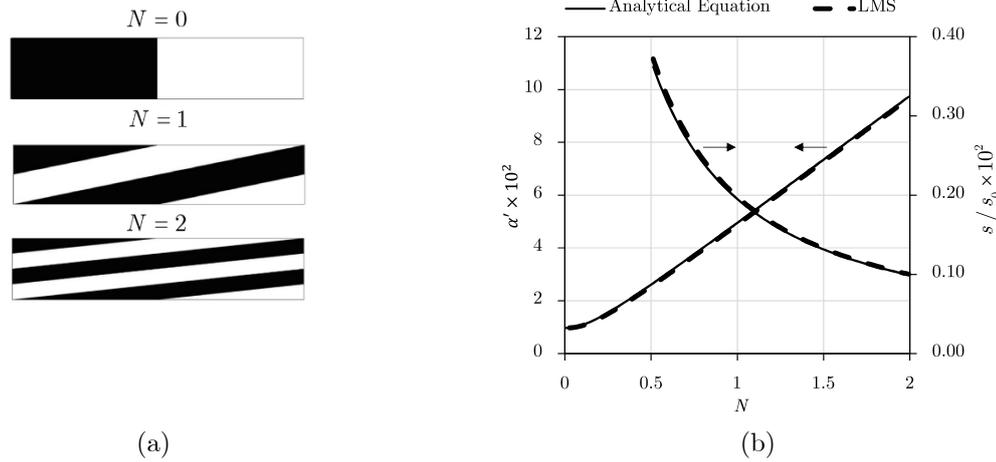
Figure 1. (a) Contour maps of 2D CFD results at the initial time ( $N = 0$ ), after one ( $N = 1$ ) and two turns ( $N = 2$ ); (b) striation thickness evolution and interfacial area growth calculated from LMS and analytical equations.
