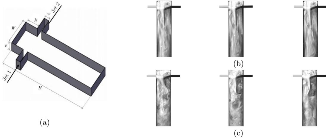
Figure 7. (a) Sketch of T-Jets mixers and respective dimensions; (b) PLIF images for mixing of two dissimilar with a viscosity ratio of 3 using geometry W6w1e4 at (b)  $Re_{H_{jet1}} = 93$  and  $Re_{H_{jet2}} = 560$ ; (c)  $Re_{H_{jet1}} = 105$  and  $Re_{H_{jet2}} = 640$ .
