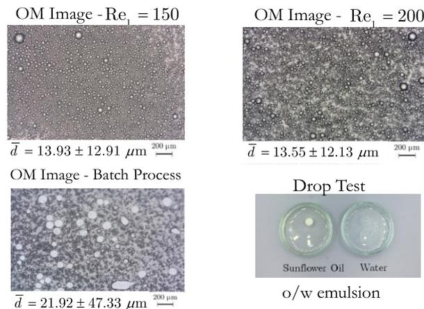
Figure 6. Optical Microscope images of emulsions produced in the continuous process for  $Re_{oil} = 150$  and  $Re_{oil} = 200$ , in a batch process, the respective droplet diameter and photograph of the drop tests for o/w emulsions.
