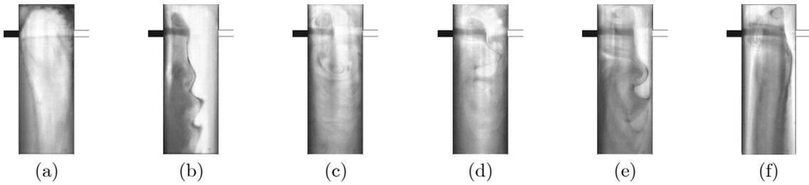
Figure 4. PLIF images for a viscosity ratio 5 at  $Re_2 = 70$  using Chamber 1 and at (a)  $Re_1 = 168$ ; (b)  $Re_1 = 243$ ; (c)  $Re_1 = 250$ ; (d)  $Re_1 = 289$ ; (e)  $Re_1 = 303$ ; (f)  $Re_1 = 350$ .
