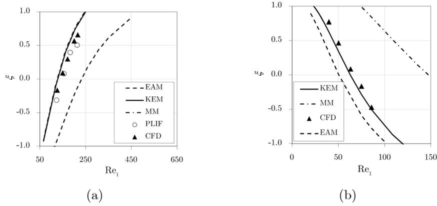
Figure 5. Dimensionless IP point determined from EAM, KEM, MM, CFD results and PLIF data for the mixing of dissimilar fluids with viscosity ratio 5 and (a) density ratio of 1 and  $Re_2 = 45$  and (b) density ratio of 10 and  $Re_2 = 45$ .
