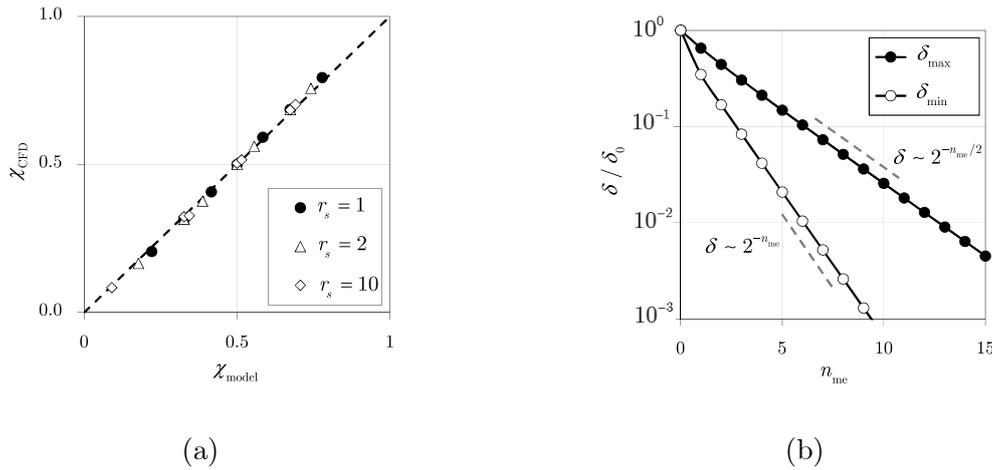
Figure 8. (a) Parity plots comparing the interface positions obtained from the analytical model and the CFD simulations for different values of  $r_s$  after 2 mixing elements; (b) rate of mixing scales decay for  $r_s = 1$  calculated for the thickness of the largest and smallest strips.
