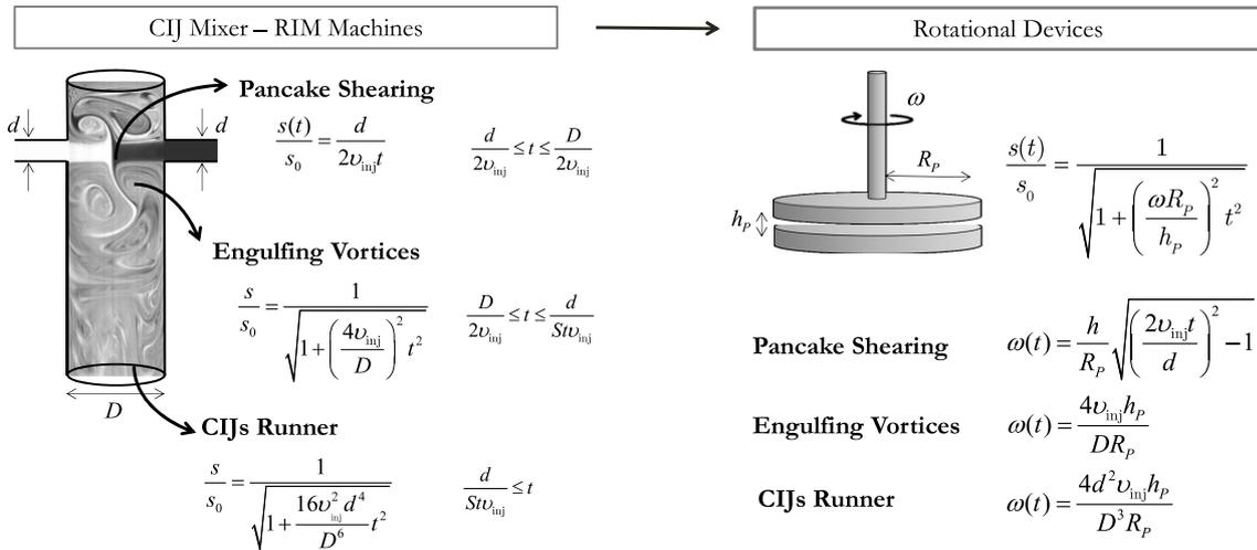
Figure 2. Mixing scales length evolution in CIJ mixers and related evolution in a plate-plate rheometer.
