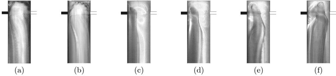
Figure 3. PLIF images for a viscosity ratio 5  $Re_2 = 50$  using Chamber 1 and at (a)  $Re_1 = 114$ ; (b)  $Re_1 = 125$ ; (c)  $Re_1 = 154$ ; (d)  $Re_1 = 154$ ; (e)  $Re_1 = 211$ ; (f)  $Re_1 = 248$ .
