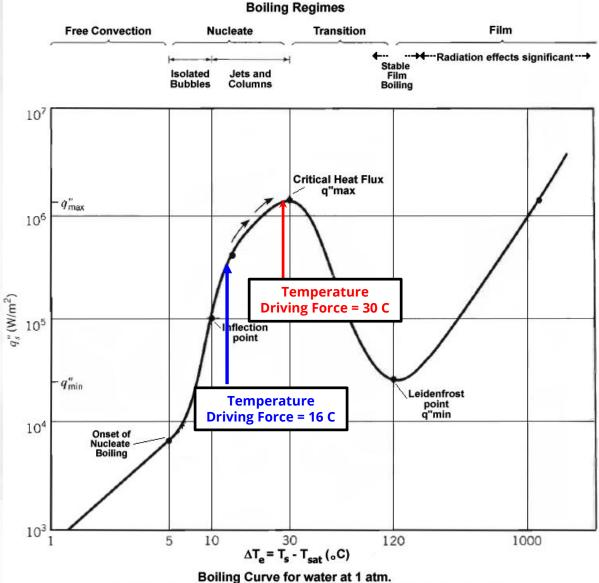
Surface heat flux q'' as a function of excess temperature  $\Delta T_e = T_s - T_{sat}$
