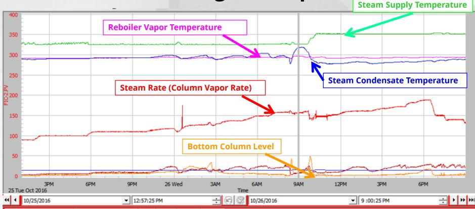
In this case, capacity increased by ~19% by operating with larger temperature driving force in reboiler
