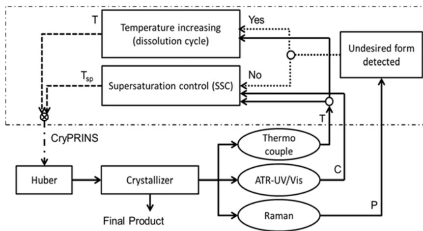
Figure 2: Schematic of the Active Polymorphic Feedback Control (APFC) approach. Raman spectroscopy is used to detect the presence of the undesired form (P) using a calibration-free approach; ATR-UV/Vis is used to measure the solute concentration (C) and perform SSC using a calibration-based approach to determine the setpoint for the temperature controller, ( $T_{sp}$ ) (17).
